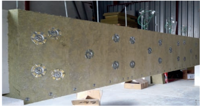
Fire protected concrete beam.
